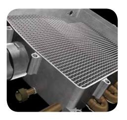
The double two-in-one heat exchanger of the Intergas Combi Compact HRE high-efficiency boiler has over a period of more than 10 years proven to be extremely reliable. Due to the separate central heating and hot water circuits there is no need for using a diverter valve and secondary domestic hot water plate heat exchanger. This eliminates a significant source of possible future component failures. Less parts means more reliability!
